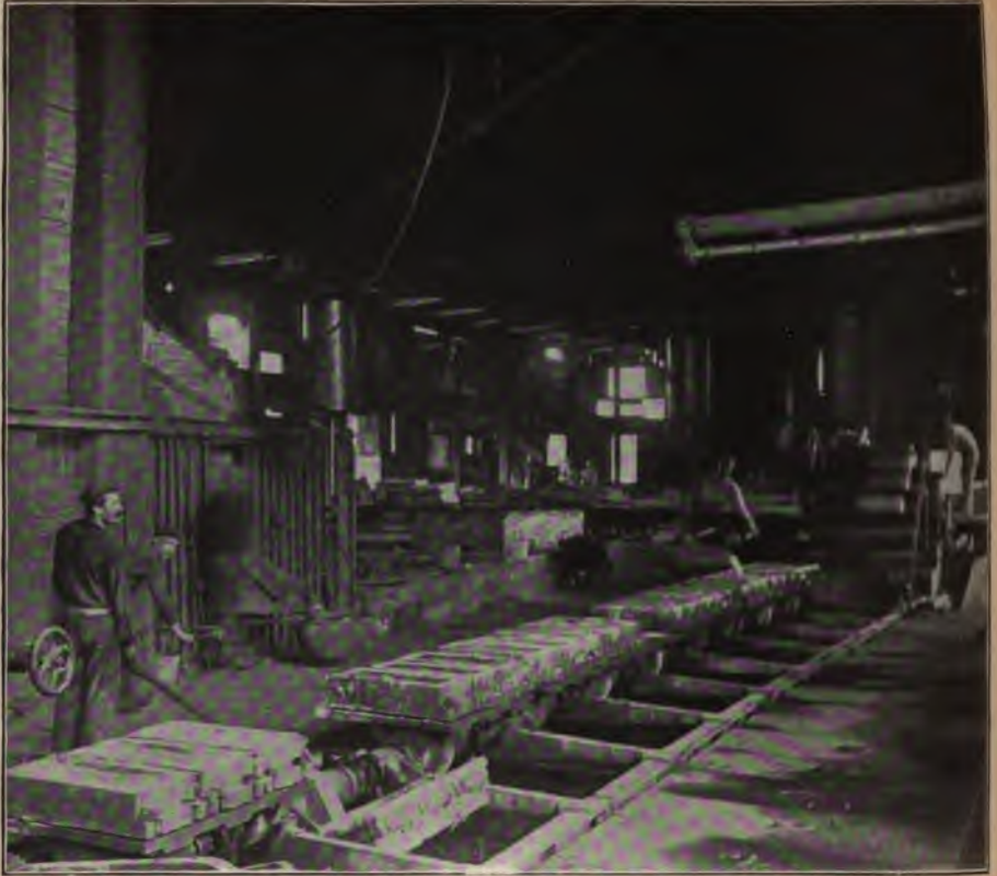
PEIRCE SEMI-MECHANICAL CASTING APPARATUS, BALTIMORE COPPER CO.'S WORKS. Showing Tapping Spout, Ladles, Tipping Molds, and Water Bosh.
